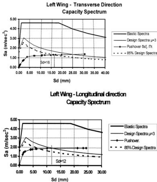
**Fig. 6** Case Study-National Library in Athens. General view of the complex; pushover analysis in transverse direction; pushover analysis in longitudinal direction.
