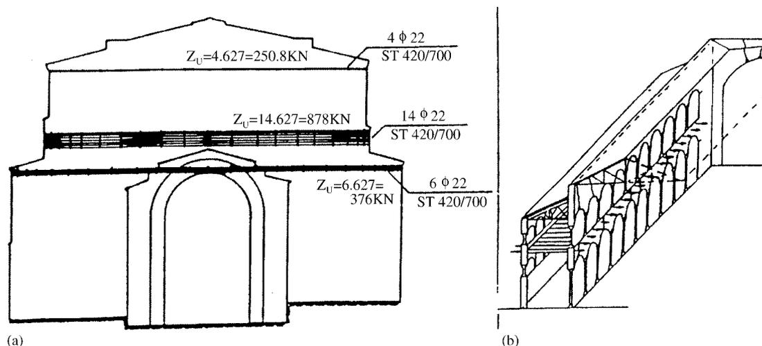
**Fig. 1** Reversible interventions: (a) prestressed rings at the base of the dome of Rotunda, Thessaloniki; and (b) improvement of the diaphragm action at the arches of Acheropoieitus church, Thessaloniki.
