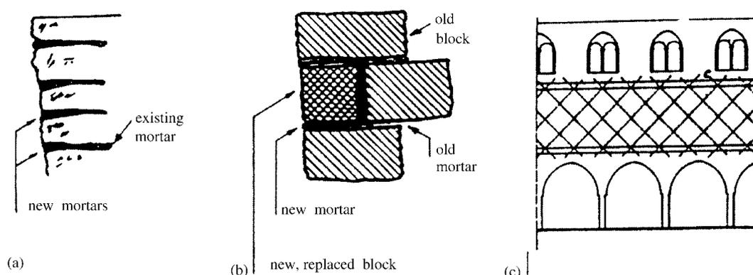
Fig. 2 Irreversible repairs: (a) deep-rejointing; (b) re-bonding; and (c) reinforcement of a colonnade (Reticolo cementato).
