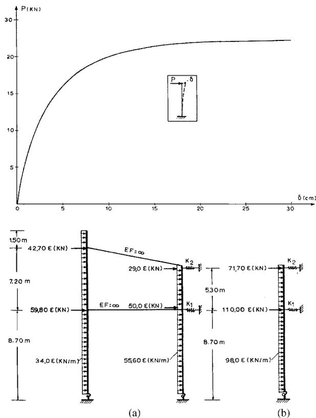
**Fig. 4** Push-over analysis of Acheropoieitus church, Thessaloniki, Greece. Structural model and  $P-\delta$  curve.
