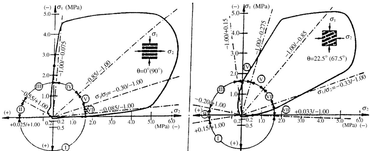
Fig. 3 Analytically determined failure envelopes of Roman Masonry (Rotunda of Thessaloniki).
